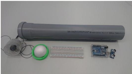
*Fig. 3: Components of the first prototype consisting of a high-temperature pipe, a hairdryer fan, a Styrofoam ball, an Arduino and an ultrasonic sensor. The breadboard simplifies the wiring of all components. A 3D-printed socket is used to attach the fan to the pipe.*
