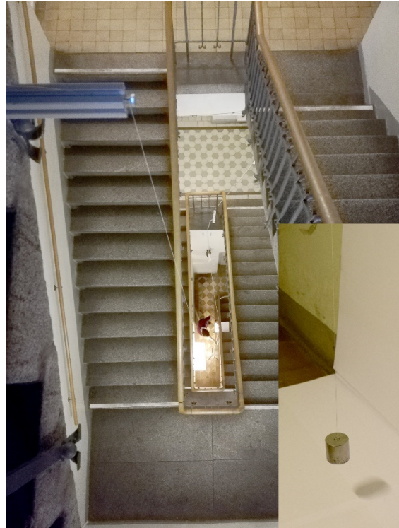
Fig. 4: Experimental set-up "Pendulum" in the stairwell of the Mollier Building
