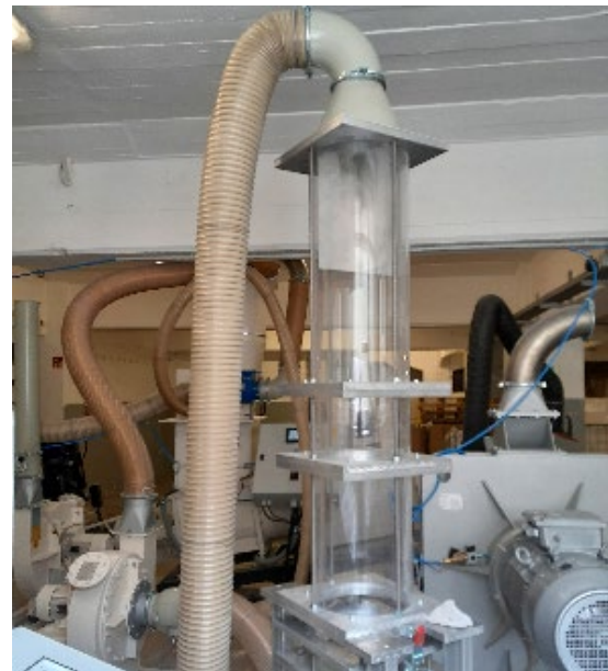
Fig. 5: Experimental setup for the production of paper fleece
