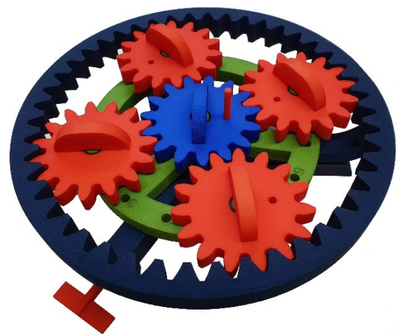
Fig. 7: Model illustrating different planetary gearboxes
