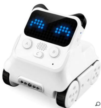
Fig. 4: A programmable CodeyRocky robot from Makeblock. The robots are movable and can be equipped with various sensors.
