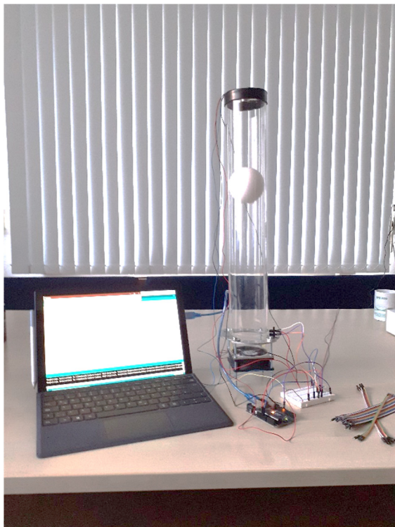
Fig. 6: Experimental set-up for the control loop with controlled system and metrological periphery.
