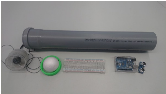
Fig. 3: Components of the first prototype consisting of a high-temperature pipe, a hairdryer fan, a Styrofoam ball, an Arduino and an ultrasonic sensor. The breadboard simplifies the wiring of all components. A 3D-printed socket is used to attach the fan to the pipe.
