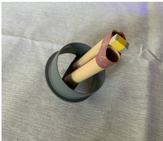
Fig. 7: Ultrasonic sensor with reduced beam angle for range extension [3.]
