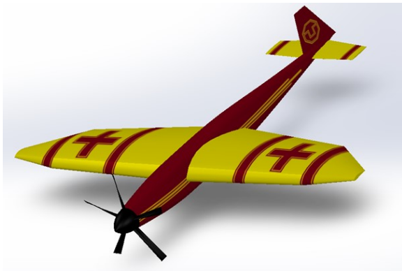
Fig. 3: sUAS before the CDR, still without the later V-position of the outer wings (cf. Fig. 6).
