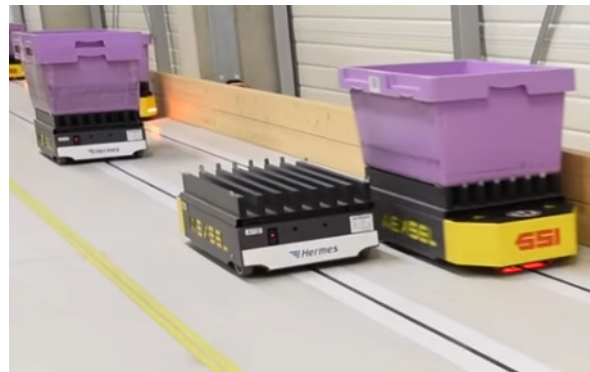
Figure 1: Example of an AGV in intralogistics [3].
