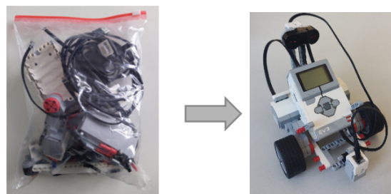
Figure 5: Hand out to perform experiments: components (left) and assembled robot vehicle (right).
