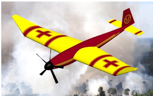
Fig. 6: Final design of the group with V-position in the outer wings to improve spiral stability.
