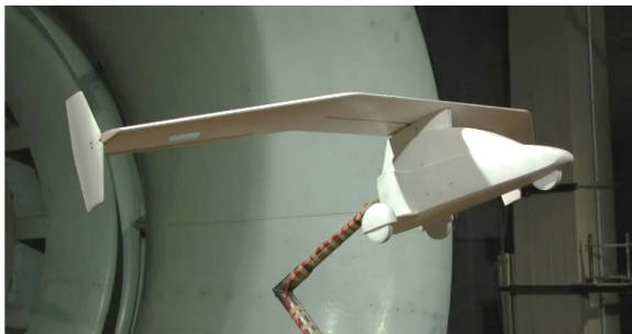
Fig. 9: Model of a tailless aircraft with a wing-span of about 2 m in the wind tunnel of the TU Dresden
