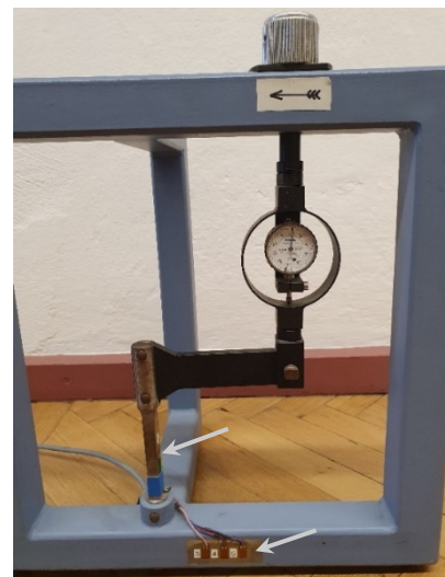
Figure 1: Structure of the laboratory course "Strain measurement". The positions of the strain gauges are marked with arrows.
