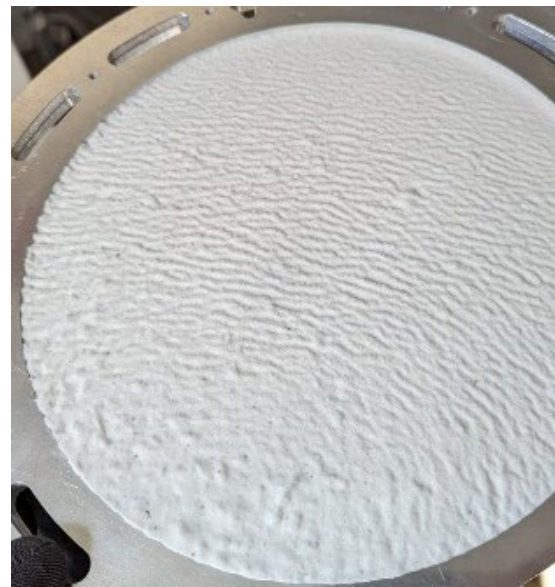
Fig. 6: Non-woven layer after completion of the deposition process
