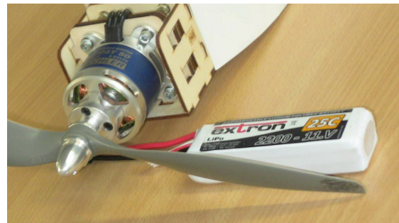
Fig. 6: Motor, propeller and flight battery from the upmarket range of model-making accessories
